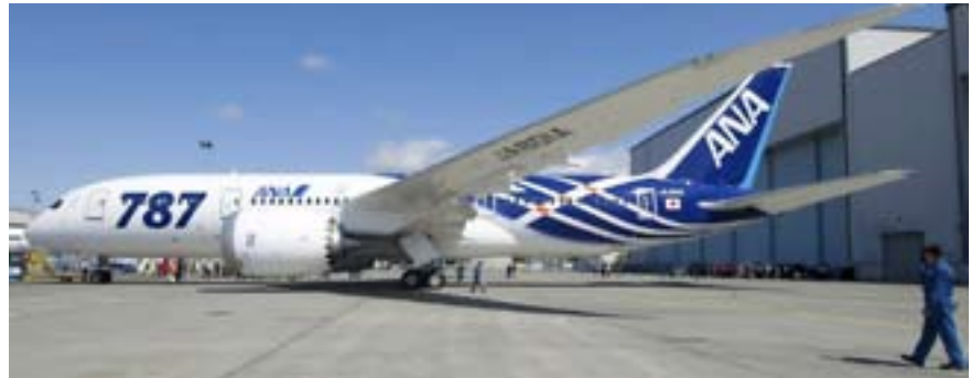
Japanese airline ANA has become the first commercial operator of the B787 Dreamliner, which has a composite fuselage. (Picture © Boeing.)
