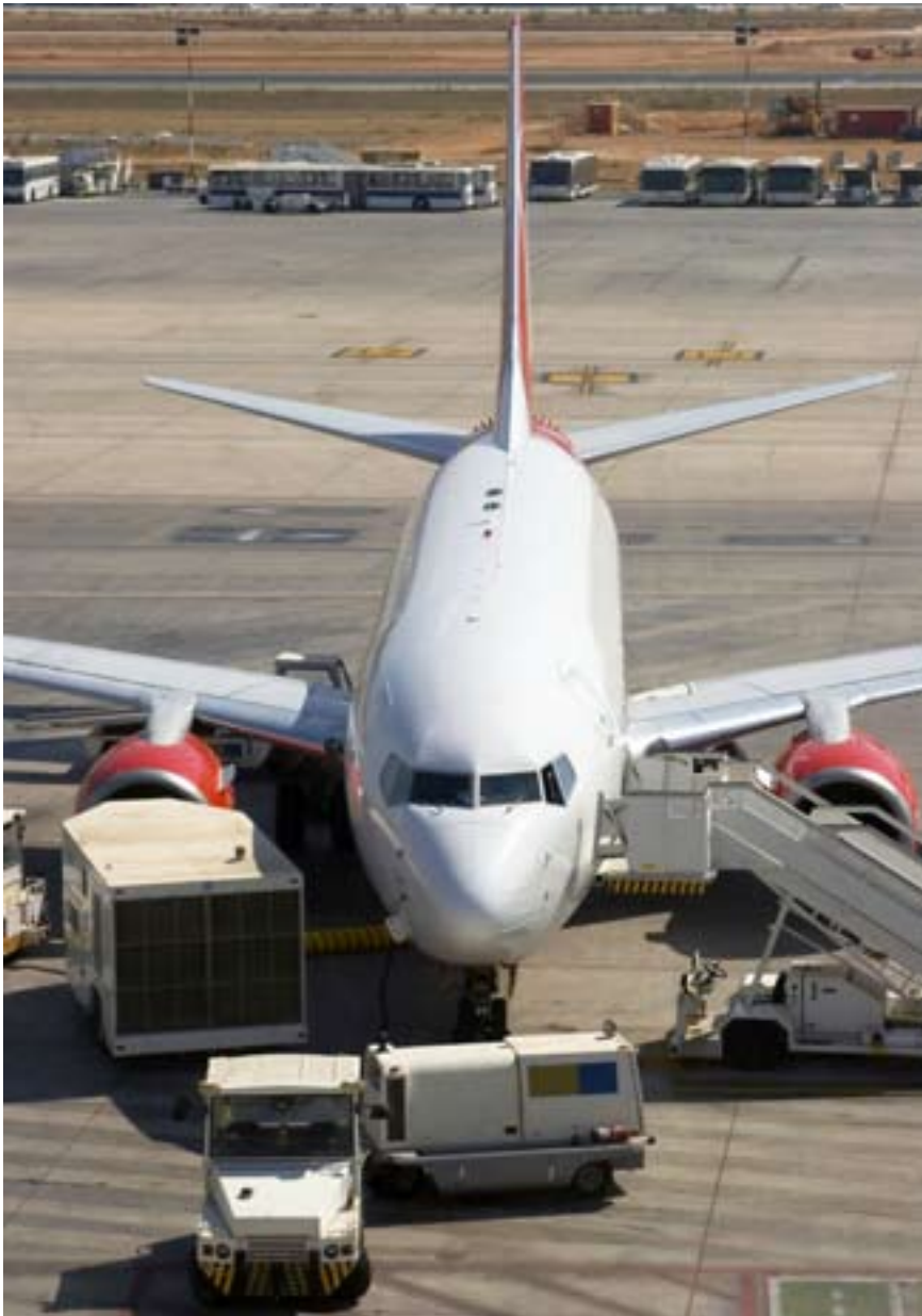
Composite fuselages are tougher than those of metal and will be more resistant to damage, but some damage will inevitably occur, especially to lower fuselage sections which are subject to impacts from numerous service vehicles. (Picture used under license from Shutterstock.com © Rob Wilson.)
